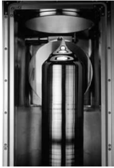
Fig. 1. Hyperpure silicon ingot in Czochralski puller—(source: SVMJ).
